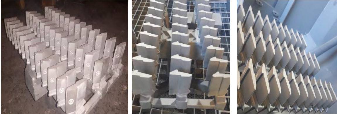
Figure 6. Castings after shakeout with improved surface
