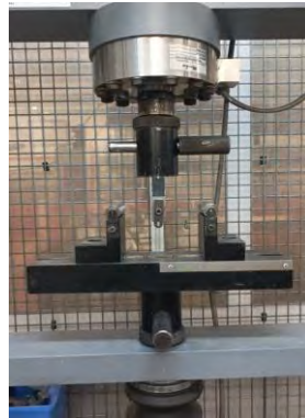
Figure 7. Picture of the 3-point bend testing machine.
