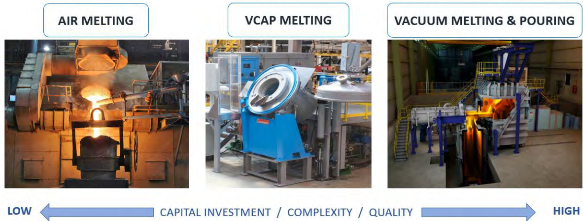
Figure 2. Sketch of VCAP technology as a mixture of air melting and vacuum melting (VIM) technologies
