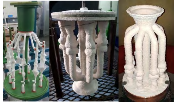
Figure 5. Cluster, shell before de-wax and after sintering
