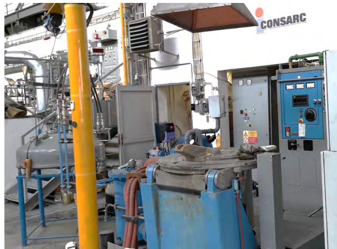
Figure 6. 175 lb (80 kg) VCAP furnace at Brno University of Technology
