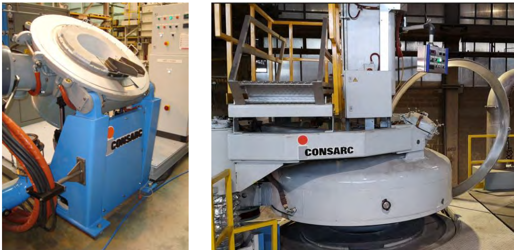
Figure 1. 80kg (left) and 1.5t (right) VCAP furnaces.
