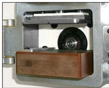
Die guide strip on platen accurately aligns molds with nozzle.
