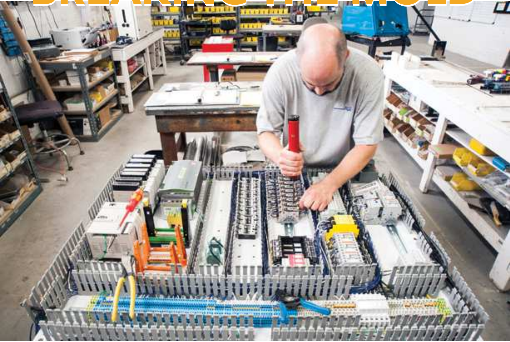
Dominic Cocco is wiring an electrical panel.
