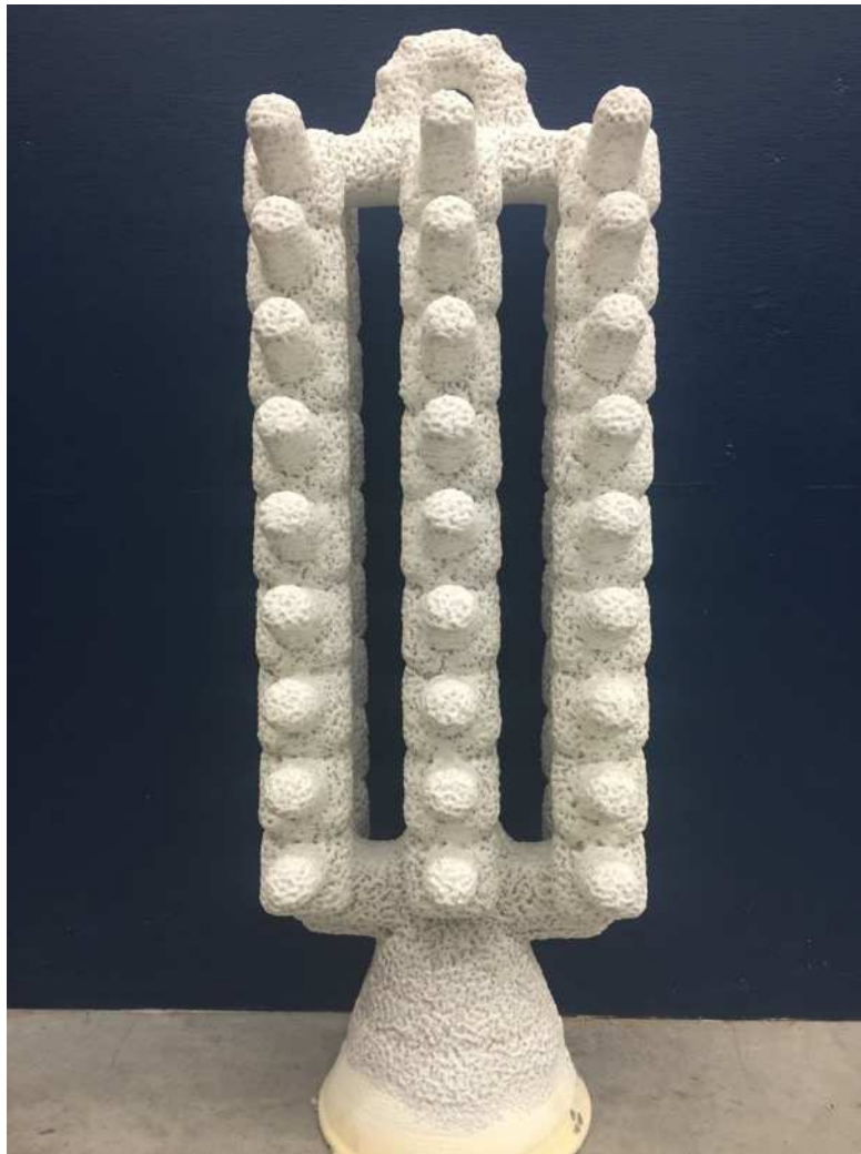
Figure 5: part # 1, 54 part tree showing bridging and shell reduction
