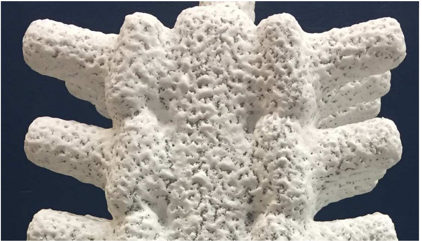
Figure 6: Part #1, Consistent shell build and bridging resulting from closer automated part spacing
