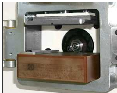
Die guide strip on platen accurately aligns molds with nozzle.
