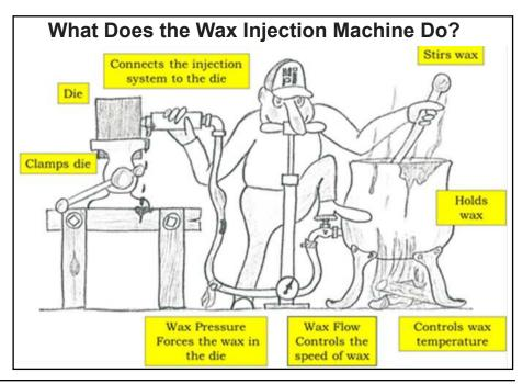
Wax Flow Control and Wax Pressure Control: Flow and pressure are controlled with either electronically controlled hydraulic servo or proportional valves. The valve's position or opening is controlled by varying the input voltage through a programmable DC driver card.
