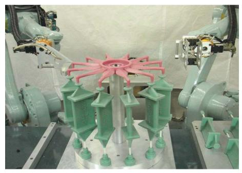
Electronically controlled robots can accurately position the patterns to create perfect position and angle for each and every single-crystal turbine blade assembly.
