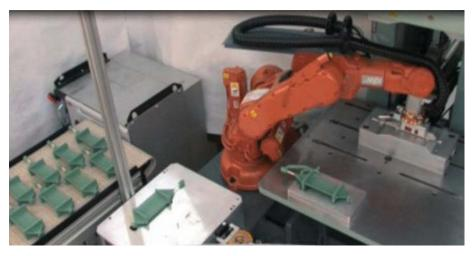
This six-axis robot can load the core, unload the pattern and perform secondary operations normally done by an operator, but without operator variation.
