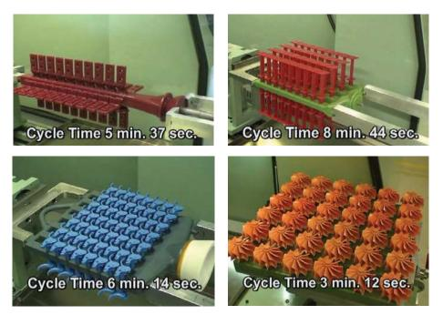
With pattern assembly using robots, more consistently accurate patterns can be included in each assemly.
