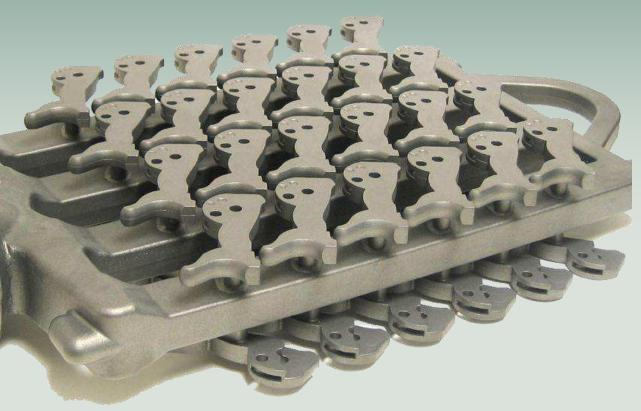
So every assembly is being produced into a single perfect casting,
