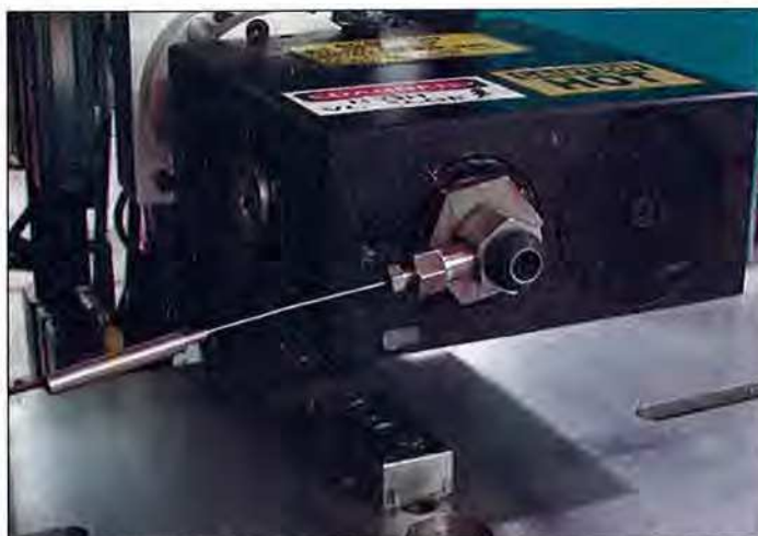
Wisconsin Precision Casting measures its wax temperature as it leaves the nozzle twice per shift.
