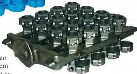
Pine Tree Castings compared the time to piece together this 40-pattern assembly when using the original manual process versus a completely automated wax cell.
