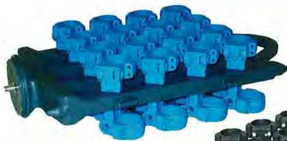
Pine Tree Castings compared the time to piece together this 40-pattern assembly when using the original manual process versus a completely automated wax cell.
