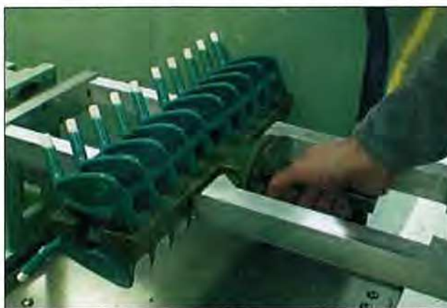
Using an automated pattern assembly system, Dolphin can rapid changeover parts eight to 10 times per day. The system runs 24 hours a day during peak demand.
