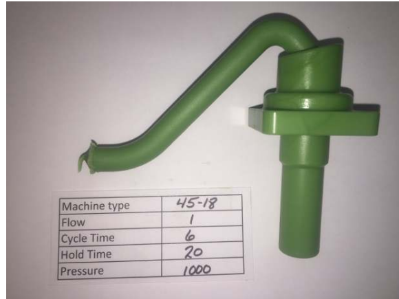
Figure 10: Sample of Short Shot picture Series Post Die Modification
