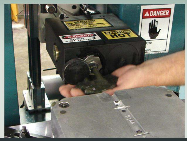
Often times after breaks, lunch, or long injection cycles, operators purge wax out of the nozzle to remove any temperature variations before they start production. If you see this being done it is a clear indication that the machine has a temperature variation.
