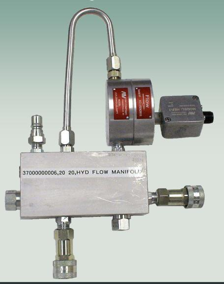
The 20/20 accomplishes this using quick-disconnects to hydraulically connect to a machine's injection cylinder,
