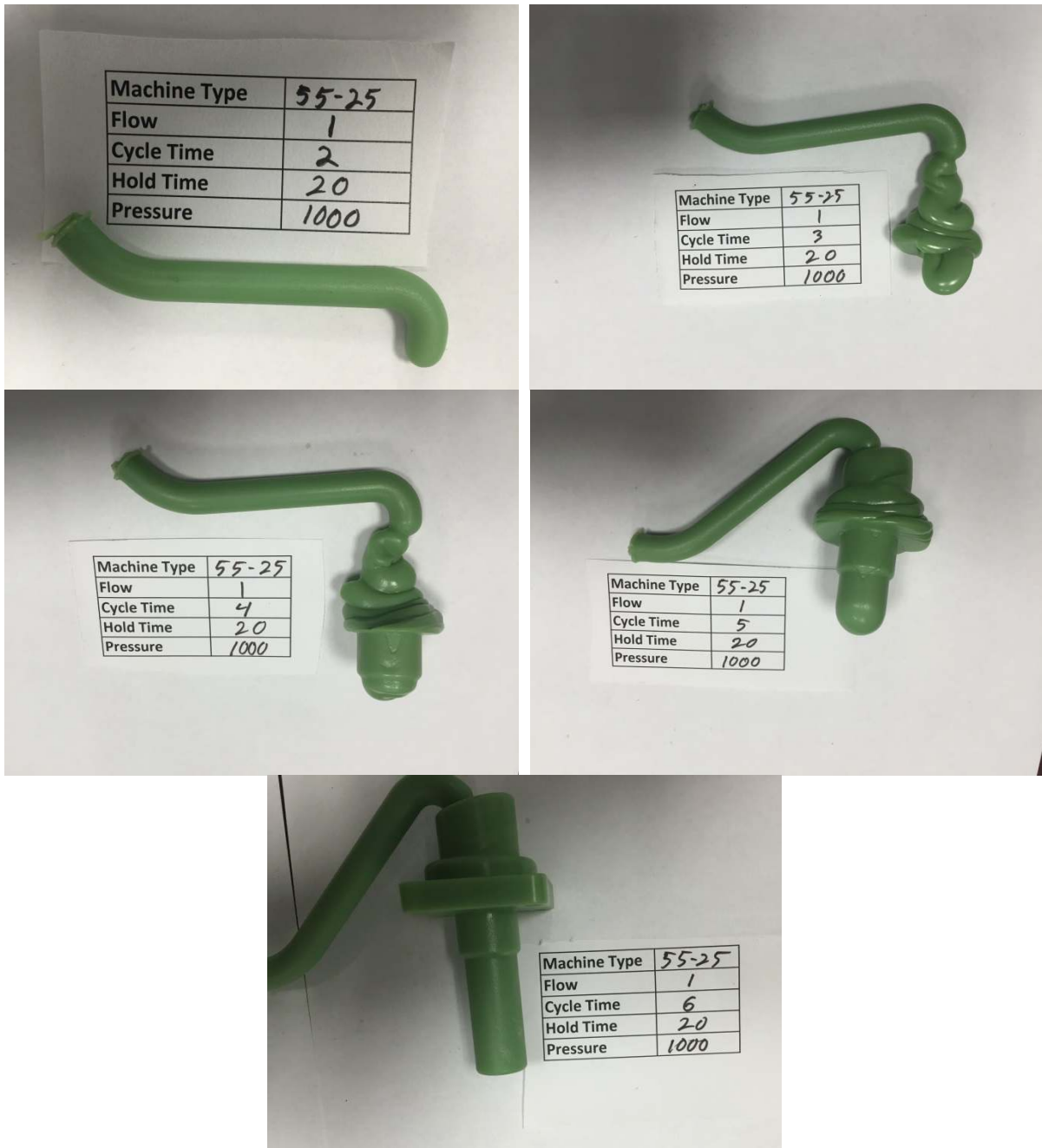
Figure 6: Sample of Short Shot picture Series
