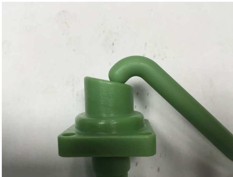
Figure 7: Picture of runner necked down
