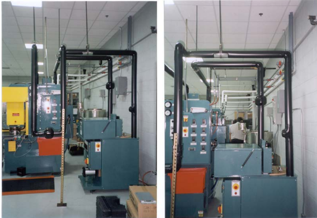
MPI's Model 94-25 Wax Preparation & Transfer Unit mounted to a rigid wax transfer line
