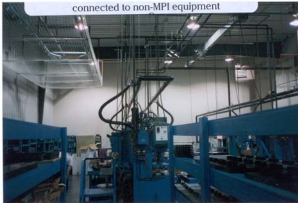
MPI's rigid wax transfer line connected to non-MPI equipment
