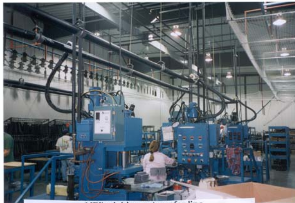
MPI's rigid wax transfer line connected to non-MPI equipment
