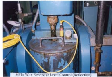
MPI's Wax Reservoir Level Control (Reflective) connected to a Jahnke press' refill port
