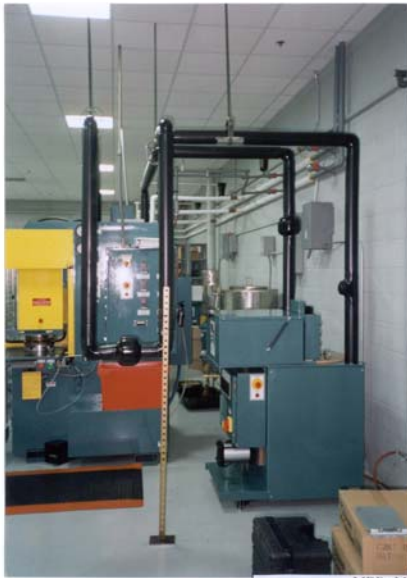
MPI's Model 94-25 Wax Preparation & Transfer Unit mounted to a rigid wax transfer line
