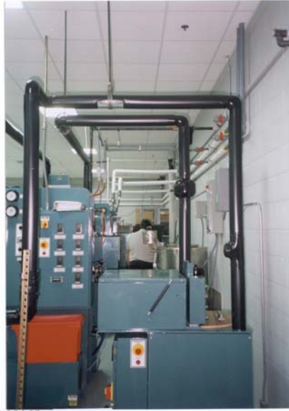
MPI's Model 94-25 Wax Preparation & Transfer Unit mounted to a rigid wax transfer line
